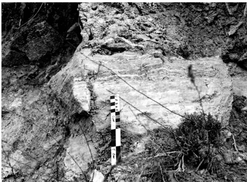
Fig. 1 - Laminitic facies in evaporitic series (Jebuc Formation) - Stana (Cluj county). It consists of a succession of gypsum laminae interlayered with clayey laminae.
