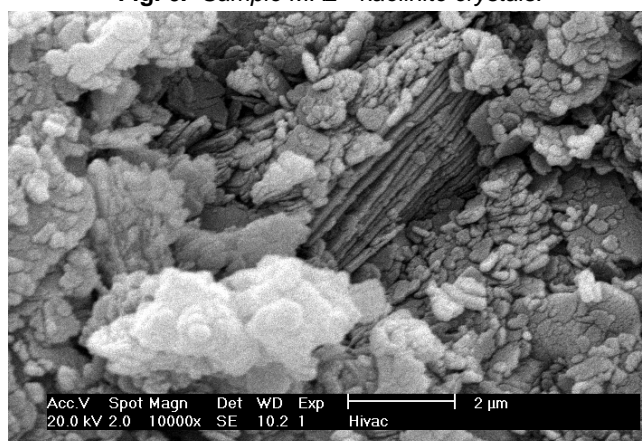
Fig. 7. Sample BOJ - kaolinite crystals.
