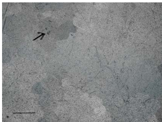
Fig. 8. Microphotograph of a pseudohexagonal siderite crystal: arrow indicates microfractures (defective zones) N+ scale bar: 1 mm.
